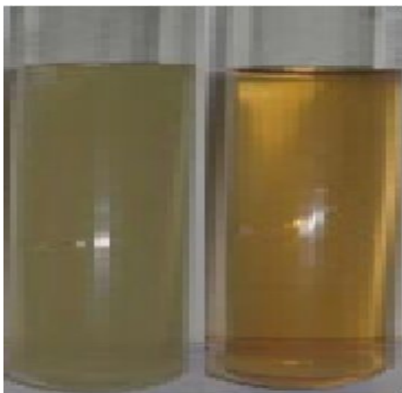
Fig.1. Aqueous solution of \text{AgNO}_3 with Senna siamea aqueous leaf extract and synthesized silver nanoparticles from pale yellow to dark brown color
