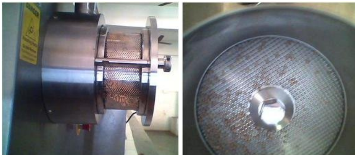
Fig.2: Assemble of the extrusion spheronization apparatus
