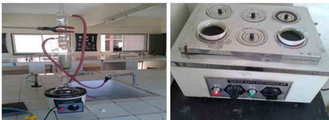
Figure No.3. Soxhlet extraction apparatus and Electronic water bath
