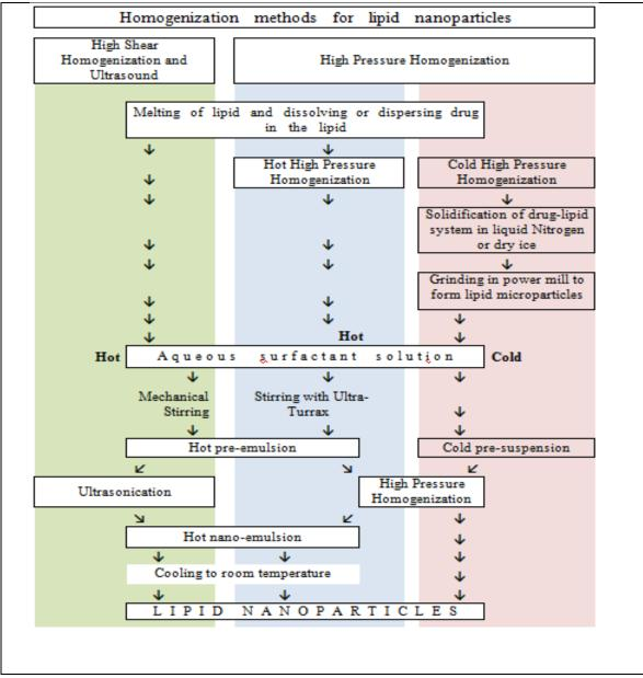
Figure 1: Schematic representation of the different homogenization techniques for the production of lipid nanoparticle.
