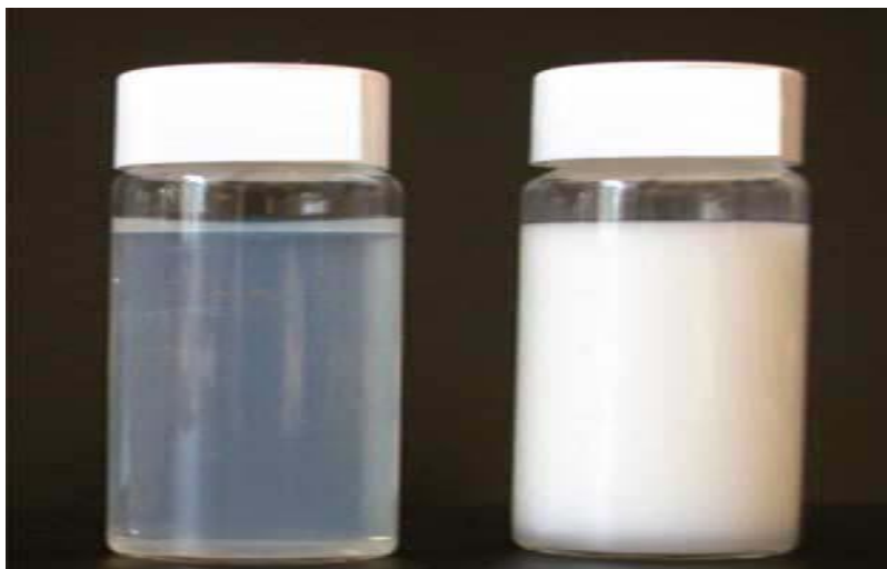
Fig.1. Nano-emulsion (left) with dia 35nm and a macro-emulsion (right) with dia 1 \mu m
